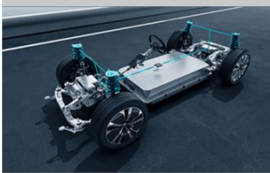
Disus-C Intelligent electrically controlled active suspension
